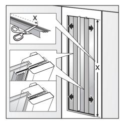
Trim the long pieces of door trim for the right and left sides to the length required X. Fix the door trim into the gap between the furniture front and the plate glass.
